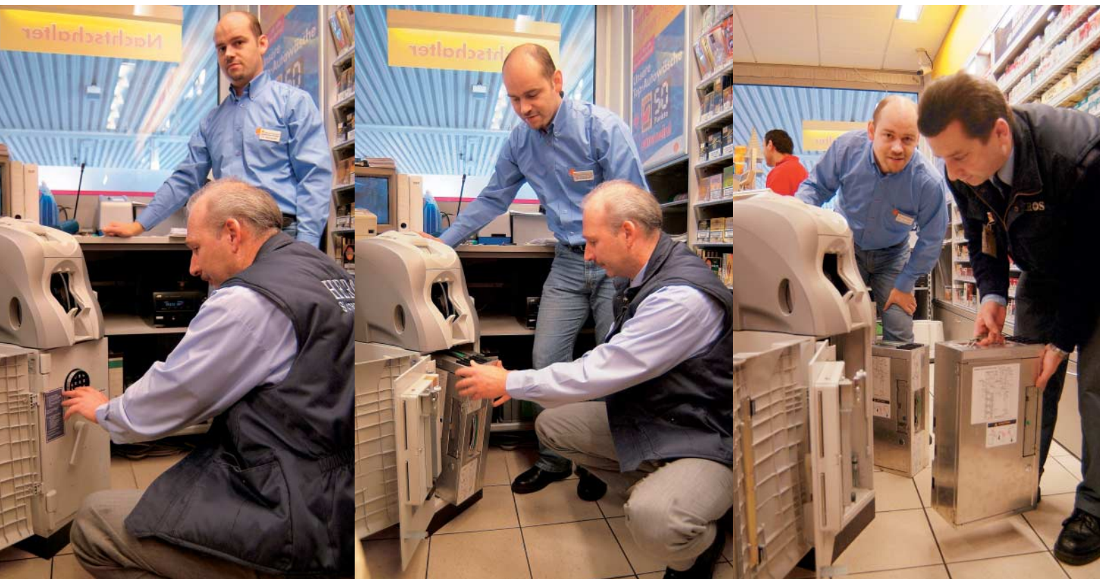
Cash handling is fast and secure: an employee of the security transport company opens the door of the safe, removes the filled cash cassette and replaces it with an empty one. The till drawer remains empty, offering no opportunities for thieves or robbers.
